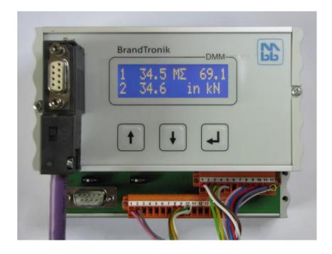
Processor based, modular structured, hybrid multichannel measuring system for transducers in straingauge technics.
